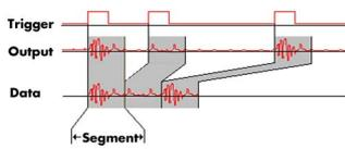
The Multiple Replay mode allows the fast output generation on several trigger events without restarting the hardware. With this option very fast repetition rates can be achieved.
