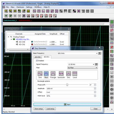
A base license of SBench 6, the easy-to-use graphical operating software for Spectrum cards, is included in the delivery. The base license makes it possible to test the card, generate simple signals or load and replay previously stored SBench 6 signals. It's a valuable tool for checking the cards performance and assisting
