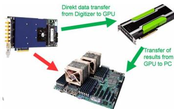
For applications requiring high powered signal and data processing Spectrum offers SCAPP (Spectrum's CUDA Access for Parallel Processing). The SCAPP SDK allows a direct link between Spectrum digitizers and CUDA based GPU cards. Once in the
