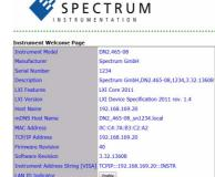
The integrated webserver follows the LXI standard and gathers information on the product, set up of the Ethernet configuration and current status. It also allows the setting of a configuration password, access to documentation and updating of the complete instrument firmware, including the embedded remote server and the webserver.
