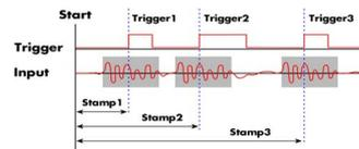
The timestamp function writes the time positions of the trigger events in an extra memory. The timestamps are relative to the start of recording, a defined zero time, ex-
