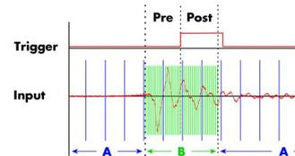
The ABA mode combines slow continuous data recording with fast acquisition on trigger events. The ABA mode works like a slow data logger combined with a fast digitizer. The exact
