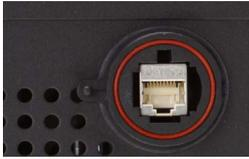
The GBit Ethernet connection can be used with COTS Ethernet cabling as well as special industrial grade Buccaneer Ethernet cables. The integration into a standard LAN allows to connect the digitizerNETBOX/generatorNETBOX either directly to a desktop PC or Laptop or it is possible to place the instrument somewhere in the company LAN and access it from any desktop over the LAN.
