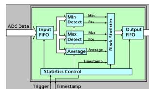
The Block Statistics and Peak Detect Module implements a widely used data analysis and reduction technology in hardware. Each block is scanned for minimum and maximum peak and a summary including minimum, maximum, average, timestamps and position information is stored in memory. The complete averaging process is done inside the FPGA of the digitizer generating no CPU load at all. The amount of data is greatly decreased as well as the needed transfer bandwidth is heavily reduced.
