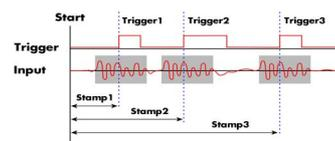
The timestamp function writes the time positions of the trigger events in an extra memory. The timestamps are relative to the start of recording, a defined zero time, externally synchronized to a radio clock, an IRIG-B or a GPS receiver. Using the external synchronization gives a precise time relation for acquisitions of systems on different locations.
