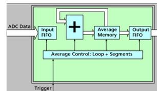
The Block Average Module improves the fidelity of noisy repetitive signals. Multiple repetitive acquisitions with very small dead-time are accumulated and averaged. Random noise is reduced by the averaging process improving the visibility of the repetitive signal. The complete averaging process is done inside the FPGA of the digitizer generating no CPU load at all. The amount of data is greatly decreased as well as the needed transfer bandwidth is heavily reduced.
