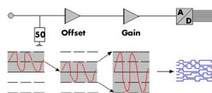
The analog inputs can be adapted to real world signals using a wide variety of settings that are individual for each channel. By using software commands one can select a matching input
