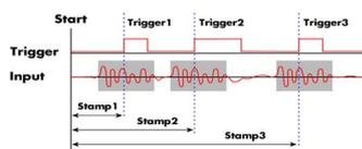
The timestamp function writes the time positions of the trigger events in an extra memory. The timestamps are relative to the start of recording, a defined zero time, externally
