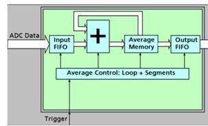
The Block Average Module improves the fidelity of noisy repetitive signals. Multiple repetitive acquisitions with very small dead-time are accumulated and averaged. Random noise is reduced by the averaging process improving the visibility of the repetitive signal. The complete averaging process is done inside the FPGA of the digitizer generating no CPU load at all. The amount of data is greatly decreased as well as the needed transfer bandwidth is heavily reduced.
