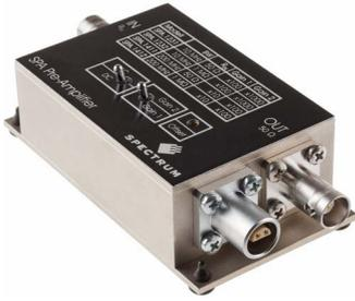
For the acquisition of extremely small voltage levels with a high bandwidth a series of external amplifiers is available. Each of the one channel amplifiers is working with a fixed input impedance and allows - depending on the bandwidth - to select different amplification levels between  $\times 10$  (20 dB) up to  $\times 1000$  (60 dB). Us-
