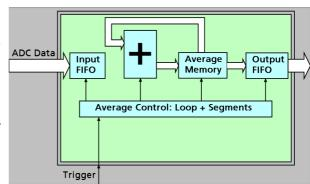
advanced trigger circuit, with very fast re-arm time, so that signals can be averaged at ultra-fast rates going as high as 5 million events per second.
