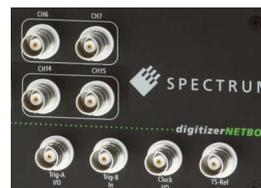
Standard BNC connectors are used for all analog input or output signals and all trigger and clock signals. No special adapter cables are needed and the connection is secure even when used in a moving environment.
