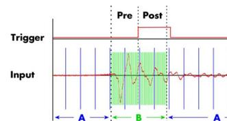
The ABA mode combines slow continuous data recording with fast acquisition on trigger events. The ABA mode works like a slow data logger combined with a fast digitizer. The exact position of the trigger events is stored as timestamps in an extra memory.
