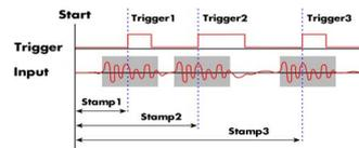
The timestamp function writes the time positions of the trigger events in an extra memory. The timestamps are relative to the start of recording, a defined zero time, externally synchronized to a radio clock, an IRIG-B or a GPS receiver. Using the external synchronization gives a precise time relation for acquisitions of systems on different locations.
