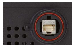
The GBit Ethernet connection can be used with COTS Ethernet cabling as well as special industrial grade Buceaneer Ethernet cables. The integration into a standard LAN allows to connect the digitizerNETBOX/generatorNETBOX either directly to a desktop PC or Laptop or it is possible
